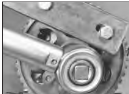
35.5 Method of tightening camshaft sprocket bolt
