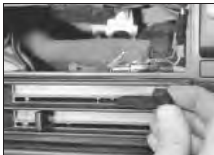
8.3a Pulling free heater/ventilation control knobs
