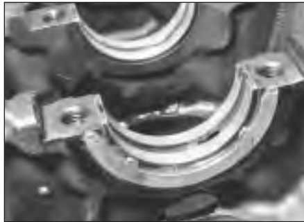
29.3 Thrustwasher location on centre main bearing
