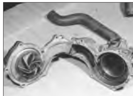
6.17 Two halves of coolant pump - 1.6 and 1.8 litre
