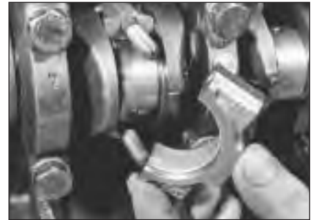
17.7 Withdrawing a big-end cap
