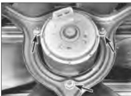
4.4 Cooling fan motor retaining nuts (arrowed)
