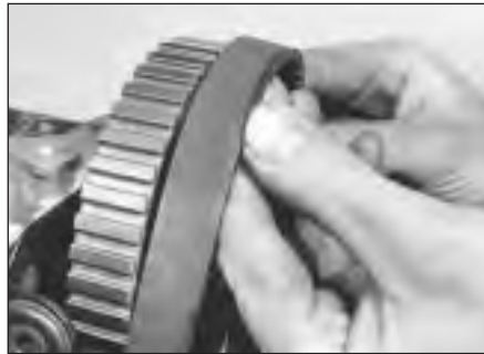
12.4 Releasing timing belt from camshaft sprocket
