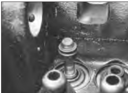
34.4 . . . then fit the new oil seal
