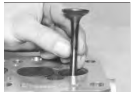
5.12 Removing a valve
