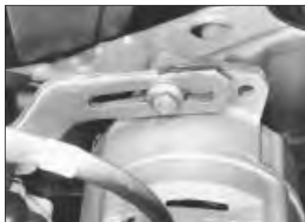
13.4a Alternator drivebelt tensioner link - 1.3 litre
