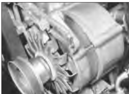
13.4b Alternator drivebelt tensioner link - 1.8 litre
