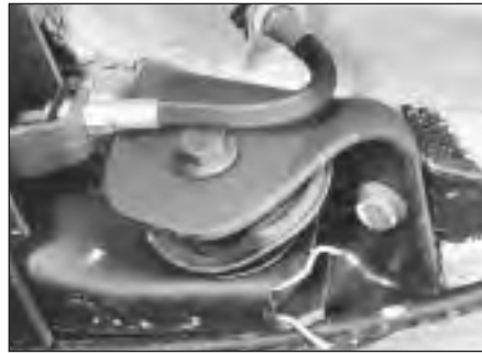
9.7 Axle beam pivot bolt head fitting position
