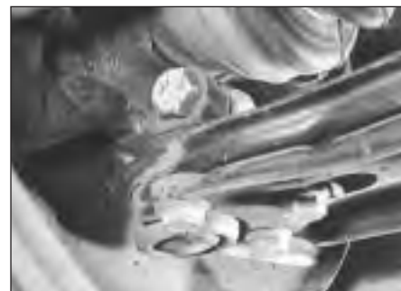
7.3 Track control arm balljoint and clamp bolt
