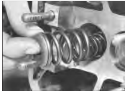
12.12b Locating valve springs and cap . . .
