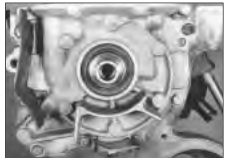
31.4 Fitted location of oil pump
