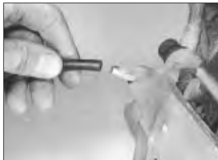
12.5 Connect bleed tube to bleed valve
