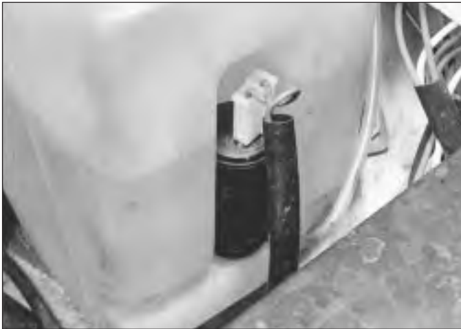
30.1 Windscreen washer pump and wire connector
