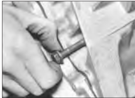
6.6a Undo securing bolts (recessed bolt shown) . . .
