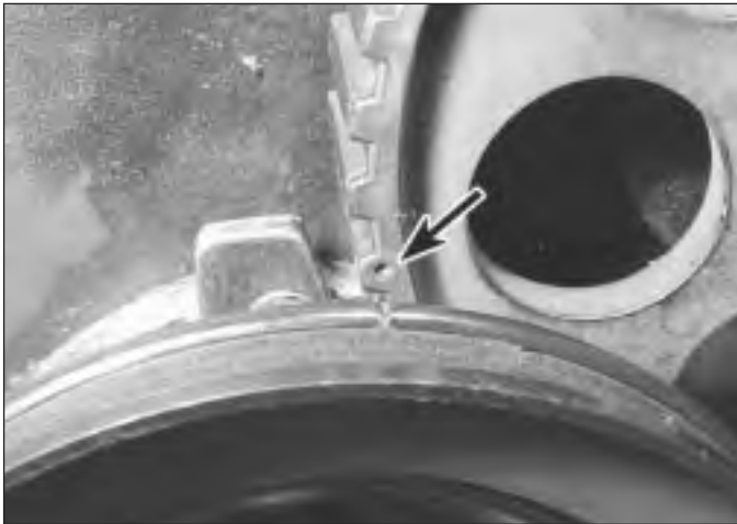
9.6 Intermediate sprocket timing mark (arrowed) aligned with notch in crankshaft pulley
