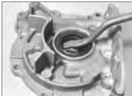
31.1 Prising out oil pump oil seal
