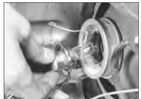
4.4 . . . and withdraw headlamp bulb
