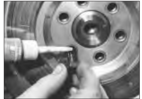
33.3 Applying liquid locking fluid to flywheel bolts
