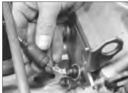
11.23c Oil pressure switch electrical connection
