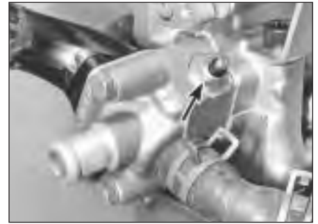
7.12 Temperature sensor (arrowed) - 1.05 and 1.3 litre
