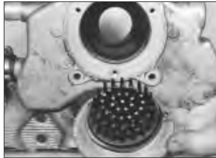
18.3b . . . and remove heater element from inlet manifold
