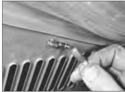
6.3 Disconnecting windscreen washer tubes from bonnet
