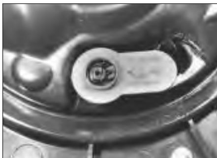
4.5 Upper view of air temperature sensor - 1.3 litre
