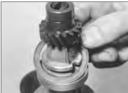
6.6b The gasket must be removed
