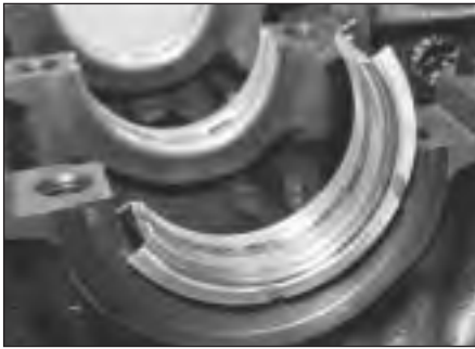
30.3a Fitting flanged type centre main bearing into crankcase
