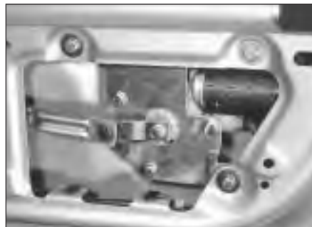
28.4b Rear wiper motor mounting in tailgate
