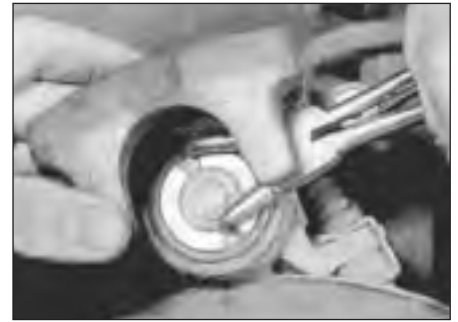
2.20b Retracting caliper piston using a pair of angled circlip pliers
