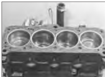
34.2 Cylinder head gasket located on block
