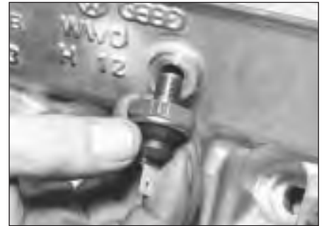
11.3 Refitting oil pressure switch
