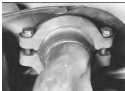
19.10 Exhaust downpipe-to-manifold flange connection - 1.3 litre
