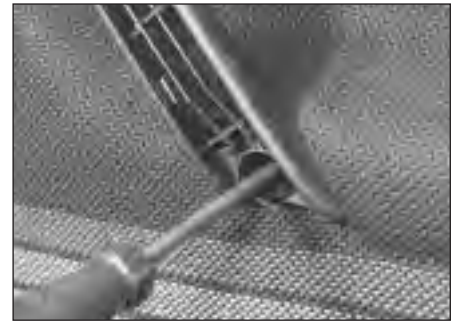
14.3b Removing door pull retaining screws
