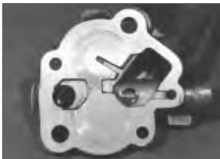
25.2 Examine face of oil pump cover for scoring
