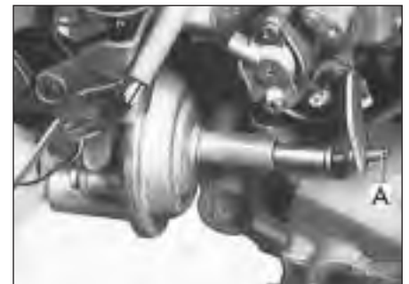
17.39b Fast idle adjustment screw (A)
