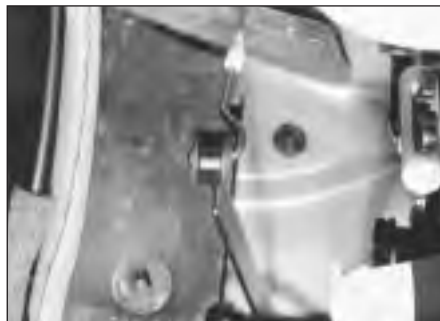
10.5 Accelerator cable-to-pedal attachment
