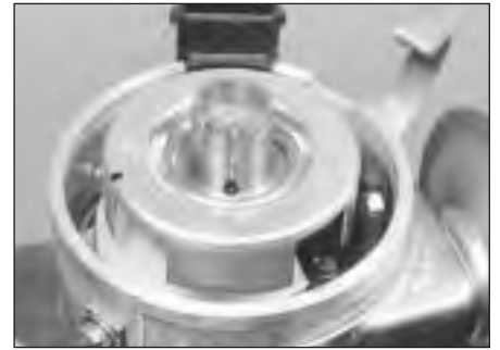
7.13 Align rotor indent with groove in shaft when refitting
