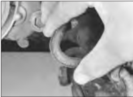
25.3a Bend each brake hose to check for cracks
