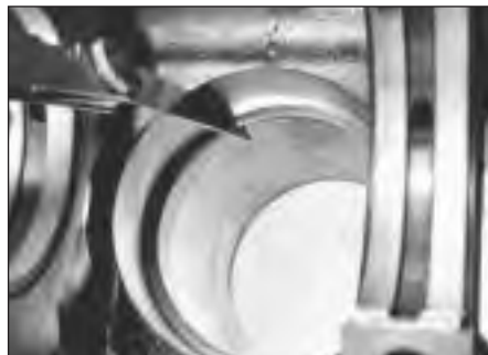
23.6 Checking piston ring gaps
