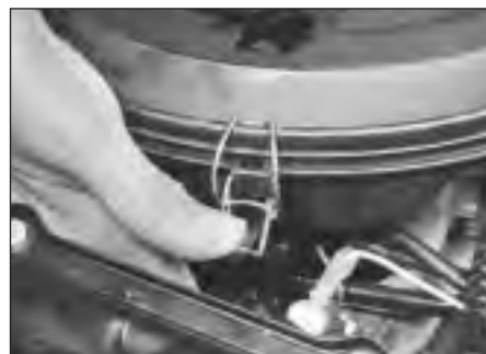
32.1 Unclip the air cleaner lid . . .
