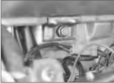
4.3 Battery retaining clamp and bolt
