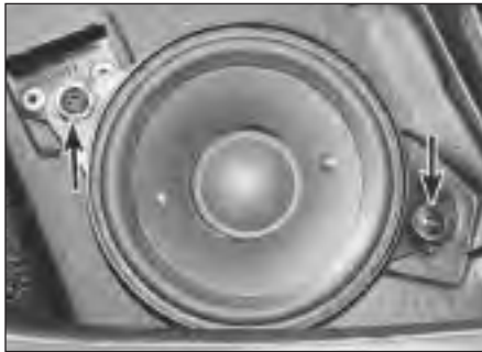
32.3 Facia-mounted loudspeaker retaining screws (arrowed)
