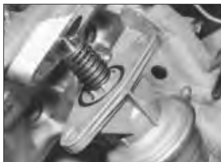
11.7a Fitting fuel pump
