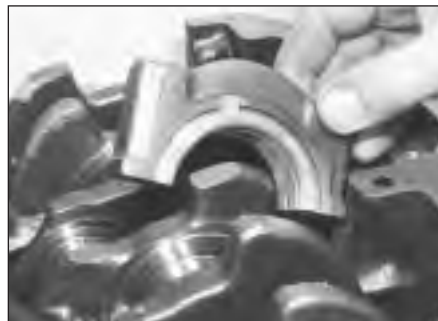
30.5 Fitting main bearing caps
