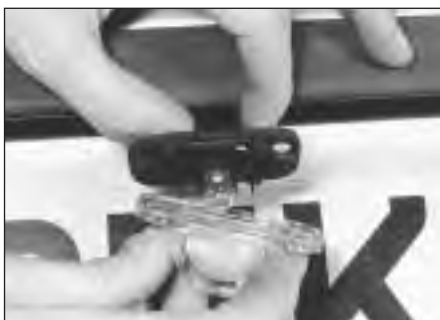
8.10 Number plate lens removal
