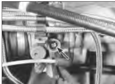
4.6 Idle speed adjustment screw location in throttle valve housing (arrowed)
