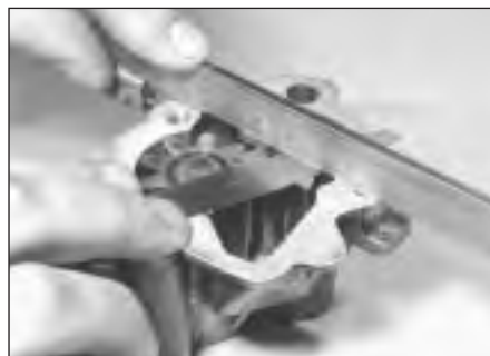
25.4 Checking oil pump gear endfloat
