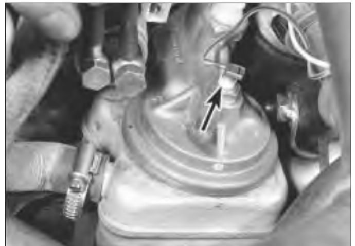
5.39 Oil temperature sender (arrowed)
