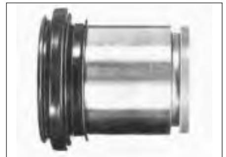
3.9 Dust seal location on caliper piston
