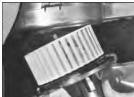
9.4 Blower unit withdrawal from housing
