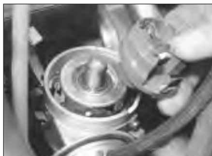
7.3a Pull free the rotor ...
