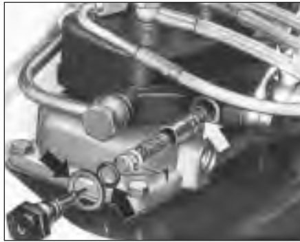
17.3 Pressure relief valve components 1 Shims Arrows indicate O-rings
