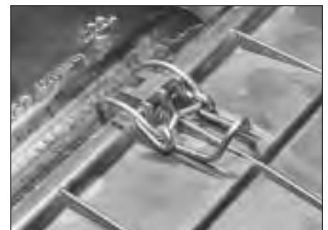
32.4a Unclip air cleaner cover . . .
