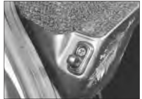
14.2 Tailgate actuated luggage compartment light switch
