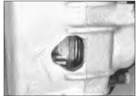
26.1 Check brake pad lining wear by viewing through inspection aperture
