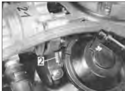
16.10 Fast idle speed adjustment screw (2)
