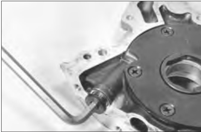
24.1a Unscrew relief valve plug . . .
