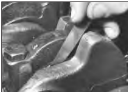
15.3 Checking crankshaft endfloat at No. 3 main bearing
