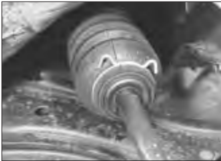
14.4 Steering tie-rod bellows and retaining clip
