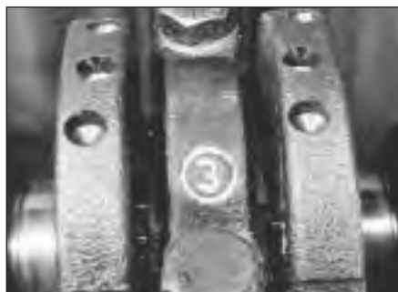
18.4 Crankshaft main bearing cap numbering
