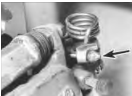
2.15 Release handbrake cable (arrowed) from caliper
