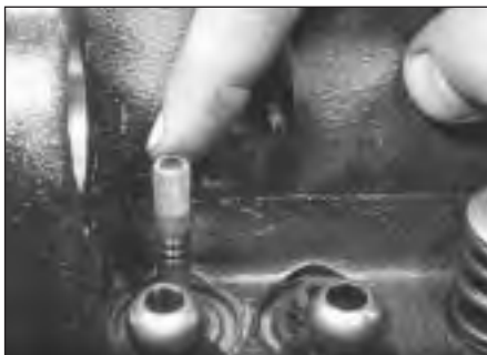
34.3 Locate plastic sleeve on valve stem . . .
