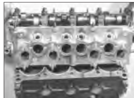
34.3a Lowering cylinder head onto block
