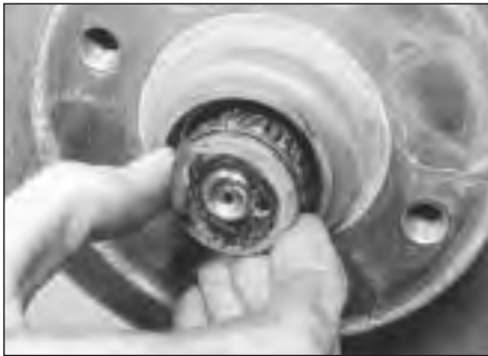
4.15 ... followed by the outer washer and bearing
