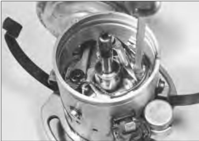
16.10b Adjusting contact breaker points gap
