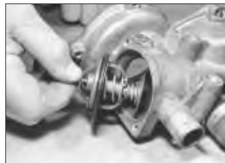
5.11c . . . then extract thermostat and seal
