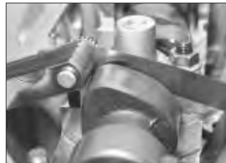
8.6 Measuring camshaft endfloat
