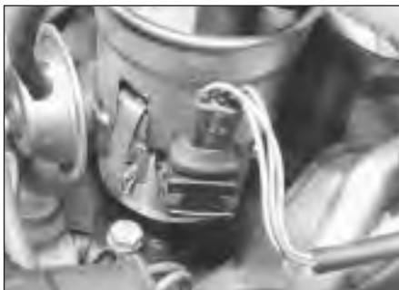
4.6a Multi-plug connection to Hall sender on side of distributor
