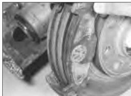
2.10 Refitting front brake pads
