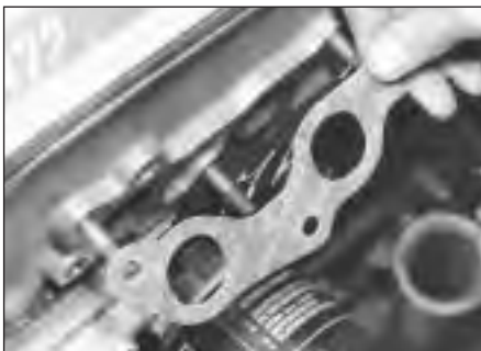
11.19 Fitting a new exhaust manifold gasket
