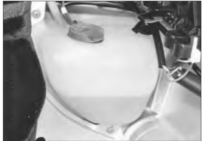
30.2 Rear window washer reservoir unit location
