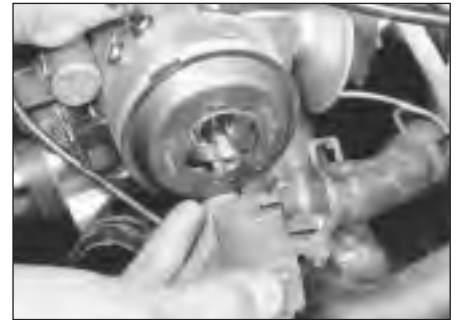
11.3 Pull off the rotor arm
