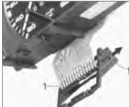
17.8b Plug housing removal from printed circuit
