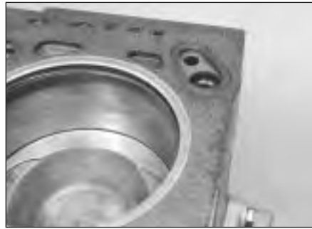
36.2 Correct fitting of cylinder head gasket
