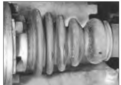
24.2 Inspect condition of each CV joint boot
