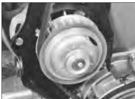
6.5 Disengage timing belt from coolant pump sprocket
