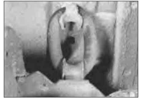
19.3 Check exhaust system mountings
