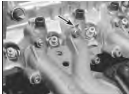
19.6 Inlet manifold-to-cylinder head securing nuts and bolts
