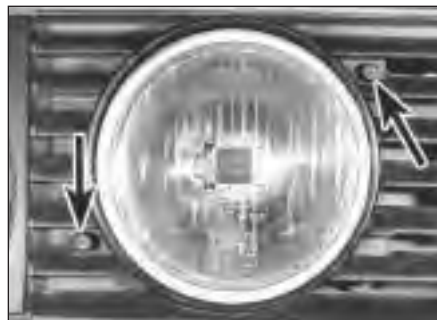
7.4 Foglight beam alignment adjuster screws (arrowed)
