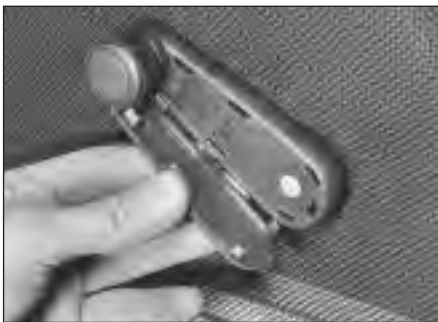
14.4a Remove window regulator handle cover . . .
