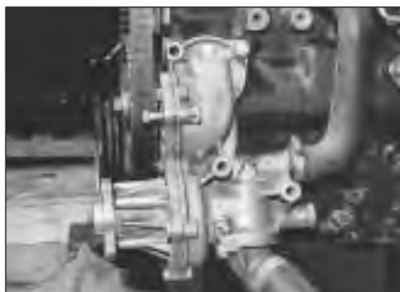
6.16 Coolant pump location (engine removed from vehicle) - 1.6 and 1.8 litre
