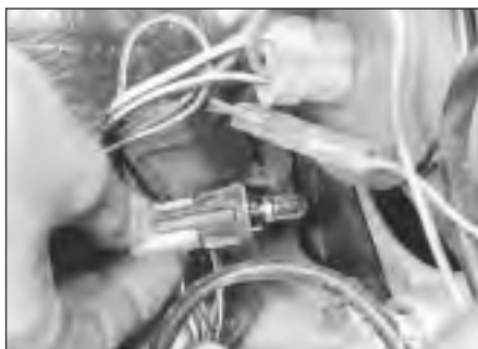
8.2 Sidelight bulb and holder removal
