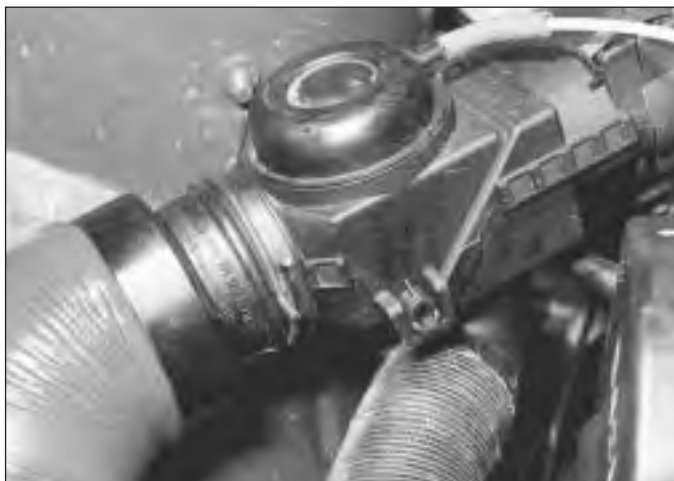
4.1 Air cleaner vacuum unit
