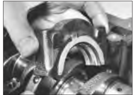
29.4 Fitting centre main bearing cap
