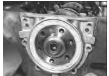
30.9 Fitting crankshaft rear oil seal and flange
