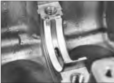
29.2 Fitting centre main bearing shell
