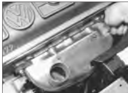
11.20 Fitting hot air shroud
