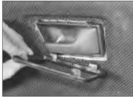
14.2 Removing door inner handle surround
