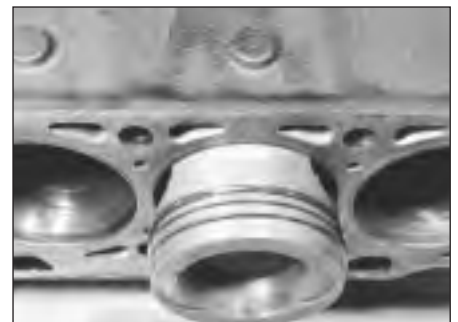
17.8 Removing a piston
