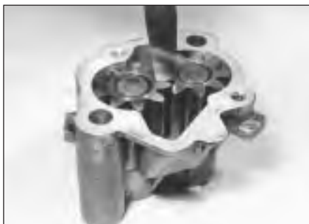
25.3 Checking oil pump gear backlash
