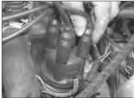
6.5 Ensure all HT lead connections are secure
