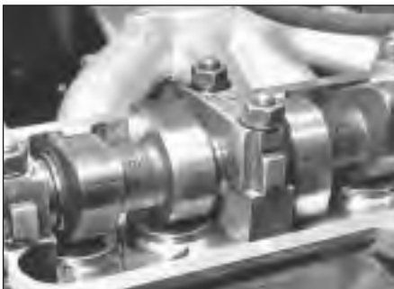
9.7b No. 1 cylinder cam lobes in valve closed position
