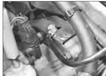
5.8c Earth strap to gearbox
