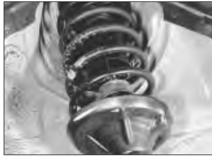
29.4 Check shock absorbers for leakage
