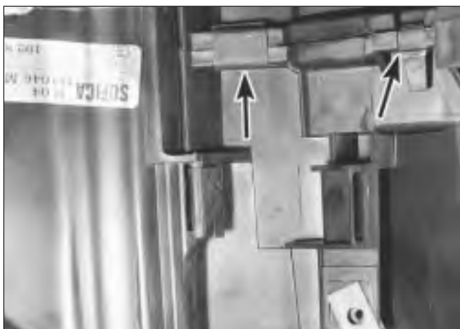
10.10 Upper-to-lower housing retaining clips (arrowed)
