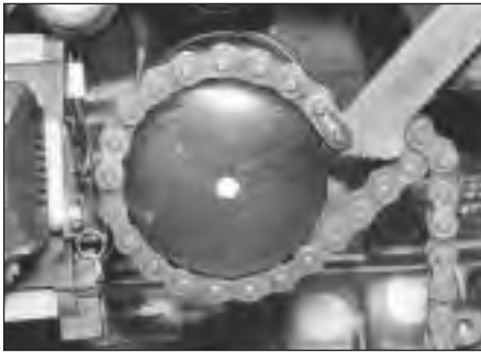
18.13 Using a chain wrench to unscrew oil filter
