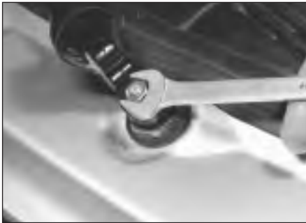
26.2 Undo wiper arm nut . . .
