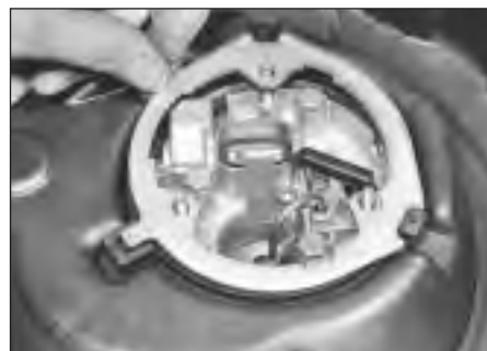
3.2 Removing air cleaner body retaining ring - 1.3 litre
