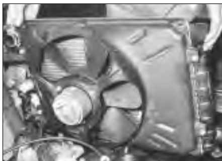
3.8 Lifting out radiator and cooling fan assembly
