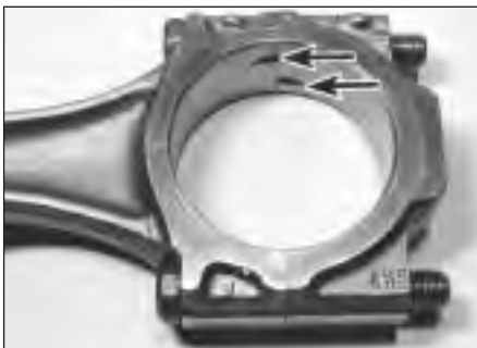
30.3 Correct location of tabs on big-end bearings (arrowed)
