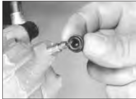
12.23 Fit bleed valve the protector cap
