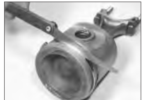
23.7b Checking piston ring-to-groove wall clearance
