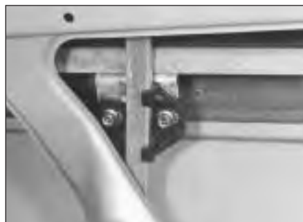
20.3b Lifting plate-to-window channel bolts
