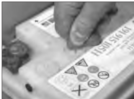
7.3a Remove battery filler caps . . .
