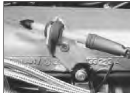
8.10 Accelerator cable adjuster and support bracket
