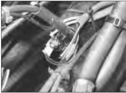
10.4 Starting motor solenoid wiring connections – 1.3 litre
