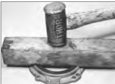
14.16 Installing new crankshaft rear oil seal
