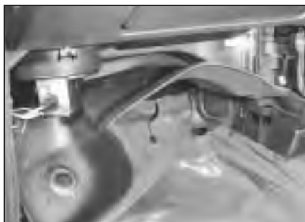
8.6b . . . and insulation sheet
