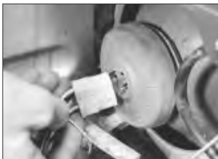
4.1 Detaching headlamp bulb connector
