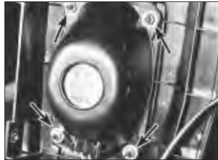
32.5 Luggage compartment loudspeaker retaining nuts (arrowed)
