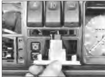
10.2 Warning lamp cluster removal
