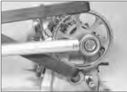
4.5 Two lengths of metal used to lock camshaft sprocket
