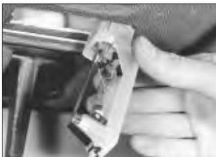
8.13b Interior light removal - 1.8 litre
