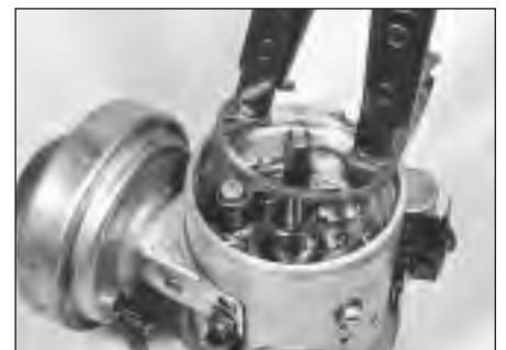
7.10b Removing bearing plate retaining ring
