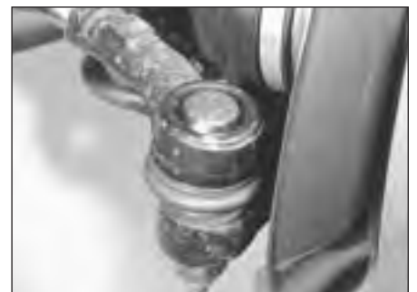
28.2 Inspect balljoint dust covers
