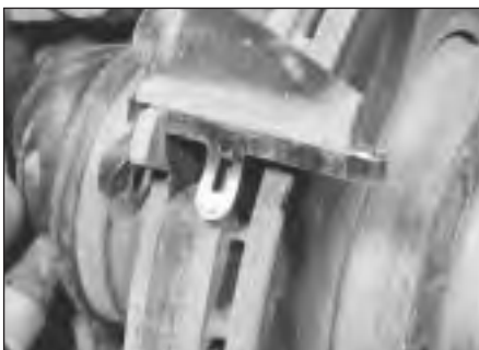
2.9 Pad retaining spring is located as shown
