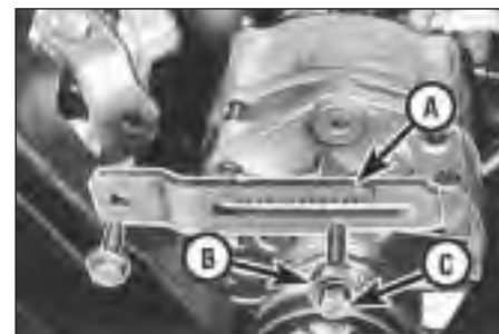
13.6 Rack type alternator drivebelt tensioner link (A) locknut (B) and adjustment bolt (C)
