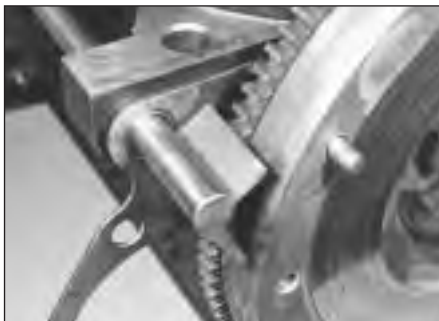
13.2 One method of holding the flywheel stationary
