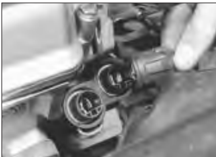
11.23b Coolant temperature switch/sender electrical connection
