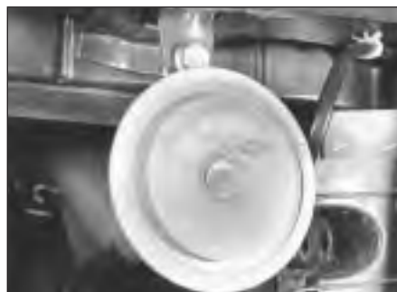
24.1a Single horn location behind front grille
