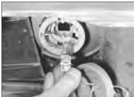
7.2 Bulb and holder removal from foglight
