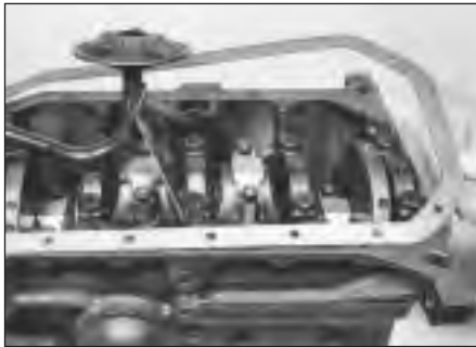
32.3 Fitting sump gasket
