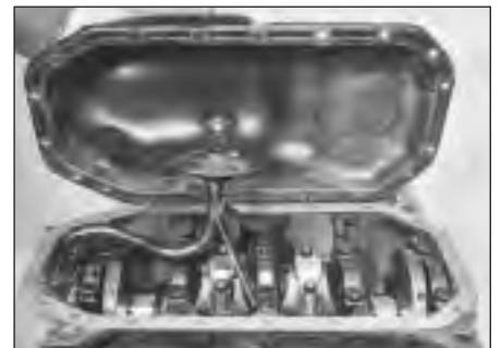
15.2 Removing the sump
