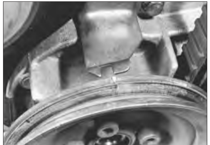
9.3b Crankshaft pulley notch aligned with TDC pointer
