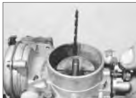
15.3a Checking choke valve gap with twist drill
