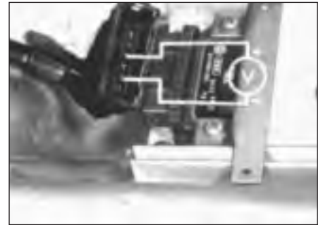
4.3 Voltmeter connection when testing ignition switch unit
