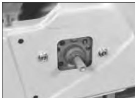
20.3a Window regulator securing bolts
