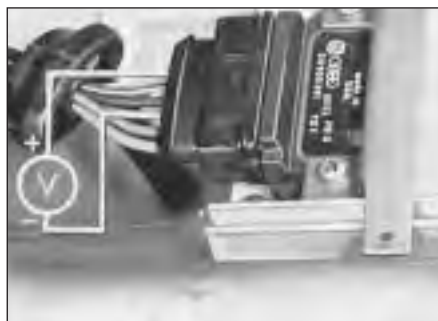
5.4 Voltmeter connection when testing Hall sender
