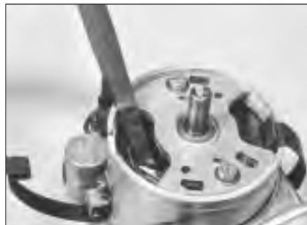
16.10a Checking contact breaker points gap
