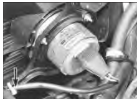
3.15 Secure fan lead with plastic clip (arrowed)
