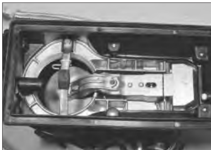
16.3 Airflow meter and fuel distributor unit (inverted)
