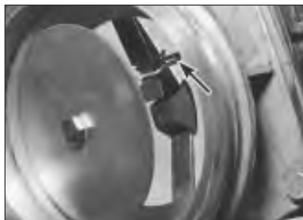
14.6 Airflow sensor plate adjustment clip (arrowed)
