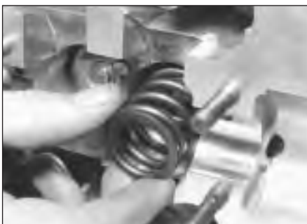
5.11a Removing an outer valve spring
